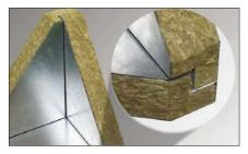
The units have a casing insulated by rockwool with a density of 110 kg/m<sup>3</sup>, which provides thermal casing insulation (Class T3(M) according to EN1886) and reduced heat losses.
